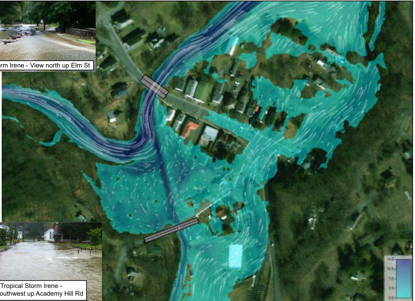
South River Walk and Watershed Tour - Stop 1. Conway center flooding. Water depth and flow paths modeled for 10-year recurrence interval event.
