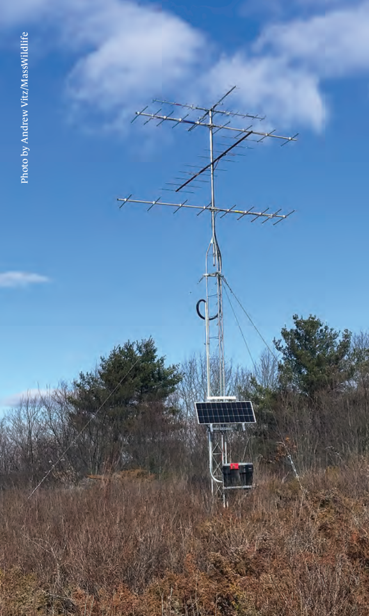
This automated radio telemetry station, located at Mass Audubon's Wachusett Meadow Wildlife Sanctuary, is part of the Motus Wildlife Tracking Network.
