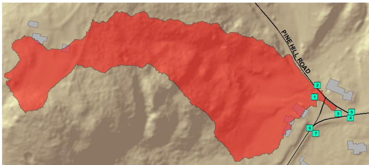
Figure 2. Estimated drainage area for culvert #3 on Pine Hill Road
