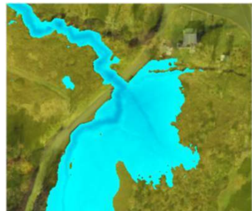
Old Cricket Hill Rd blocking floodplain
