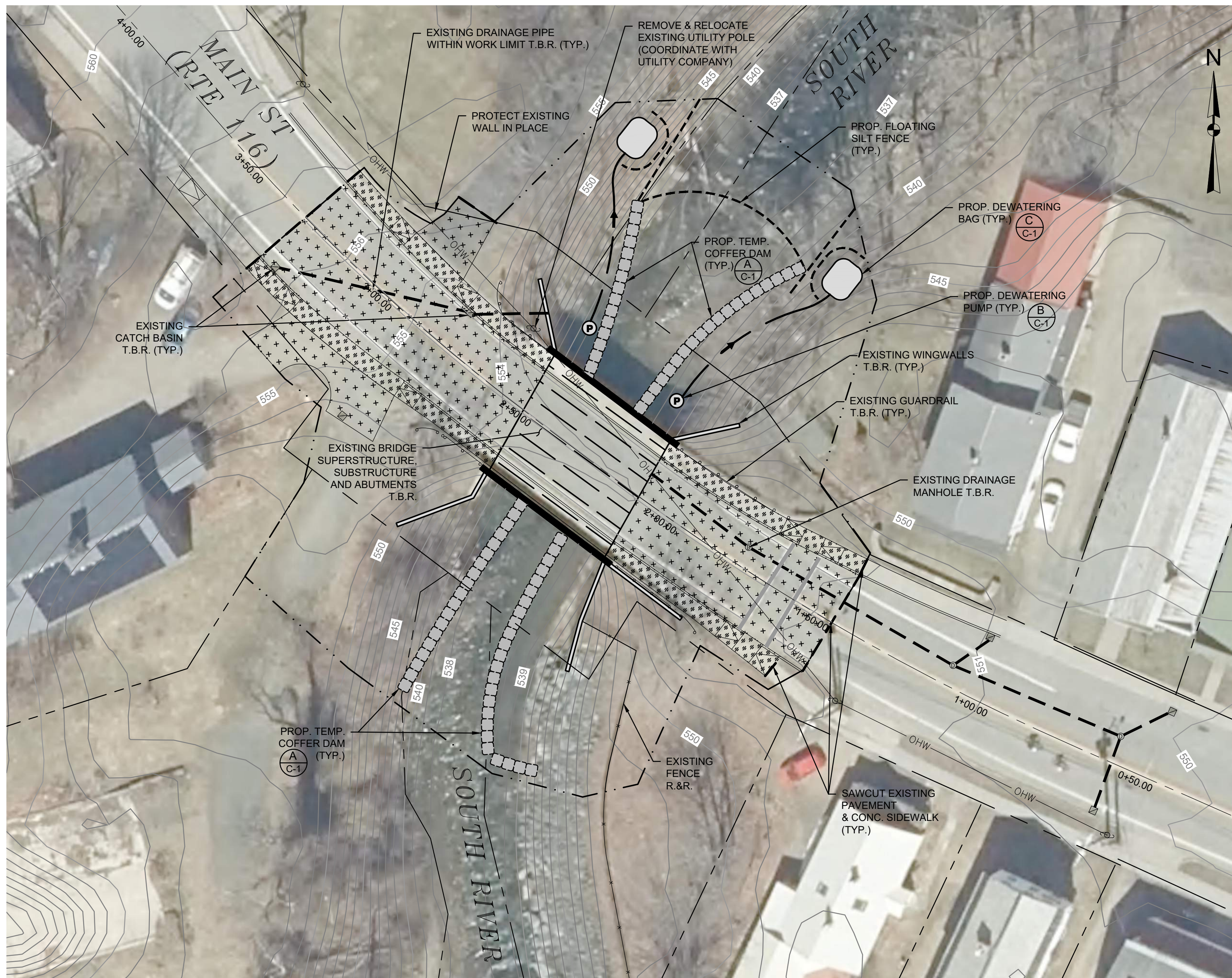
TEMPORARY WATER CONTROL, DEMOLITION AND SEDIMENT & EROSION CONTROL PLAN
